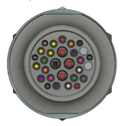
The color coded diagram above shows the wire color for each pin, keep in mind, this view is from the back of the plug (showing the wires going into the plug), so it is a reversed/mirror image from the numbered image above.
