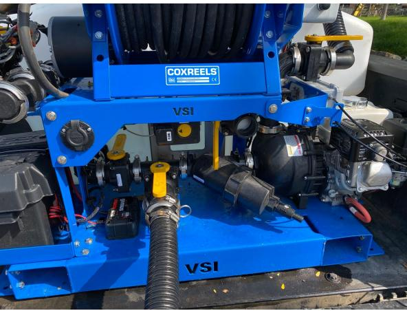
• Pump-Out Mode: Your tank must have liquid in it, your hose must be connected to the top right camlock and your valves need to be in the configuration shown when you are using the pump to transfer liquid from the sprayer to another tank outside of the sprayer. One common mistake here is that the bypass valve (top right) gets left open, which will still allow the pump-out to work, but it will be substantially slower than if it is set up properly as shown.
